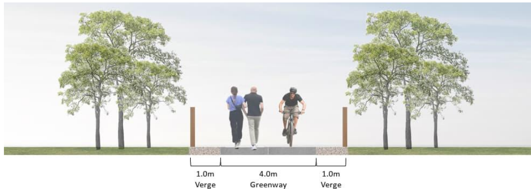
Figure 2-9 - Typical Cross Section of 6.00m Wide Greenway
